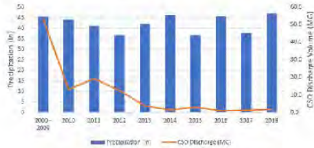
FIGURE 3-6 Auburn Sewer District 2000-2018 Precipitation vs. CSO Discharge
